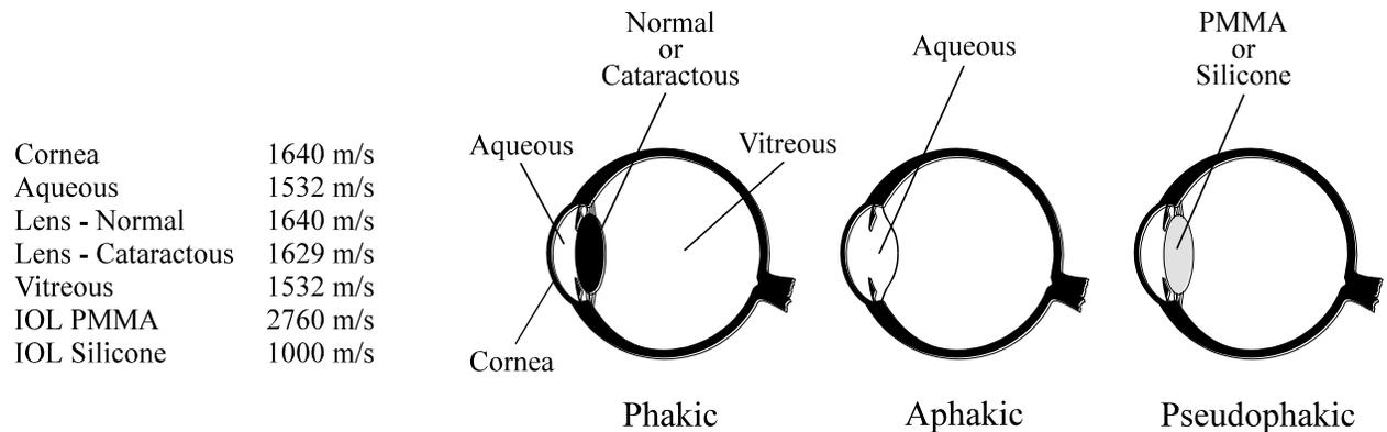
Most ophthalmic ultrasonic units use an average speed of sound of 1550 m/s for phakic eyes and 1532 m/s for aphakic eyes. The DGH 4000B is programmed to automatically use the proper speed for the eye you wish to read.
