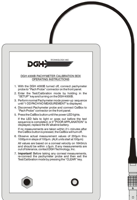
Electronic calibration box used to simulate the thickness of the cornea.
